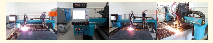
The machine FIRE BRIDGE –1500-3000(GP,G,P) is designed for cutting sheet metal with a thickness from 0.5 to 200 mm (oxygen-propane cutting). This model of the machine is possible to use for work with any type plasma sources as precision (HD) as well standard cutting quality. You can order the equipment in any variant of cutting method according of your technical demands:
